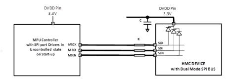
Figure 8 Reduced Impact from SPI Line Charging Uses Series Resistors on SPI Lines
