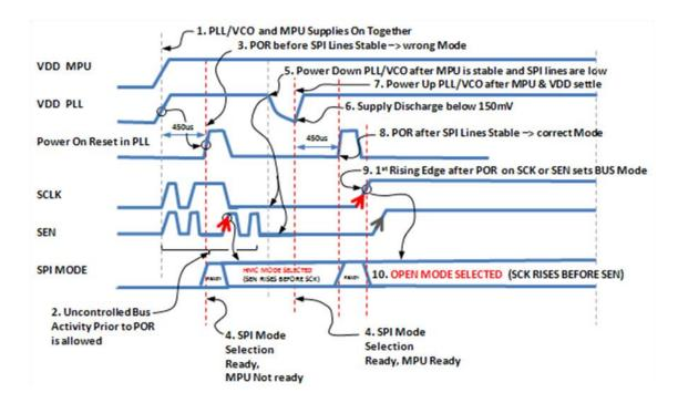
Figure 7 Mode Selection with Uncontrolled MPU on Startup
